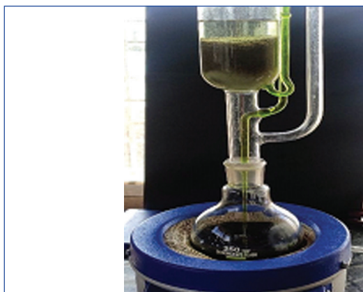
[Table/Fig-1]: Soxhlet apparatus used for the extraction of Nyctanthes arbor-tristis leaf samples with different solvents.
